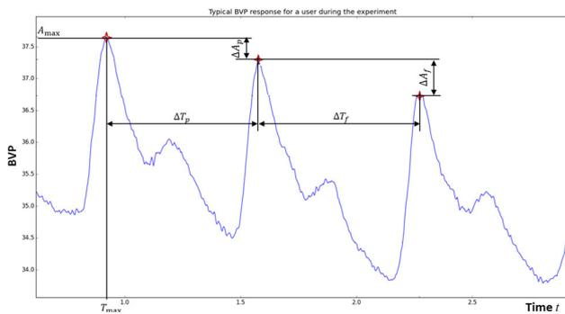
Fig. 6 An example of the BVP signal and the features of the signal
