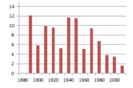
Figure 4 Overview of failure rate by installed year in region A (see online version for colours)
