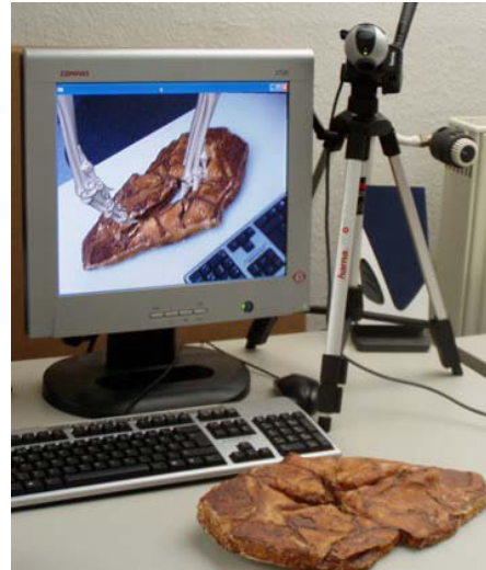
Fig. 1 Example for a screen-based video see-through display. The locomotion of a dinosaur is simulated over a physical foot-print [3].
